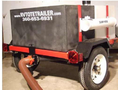
Hose carrier with 10' dump hose attached to dump valve.
