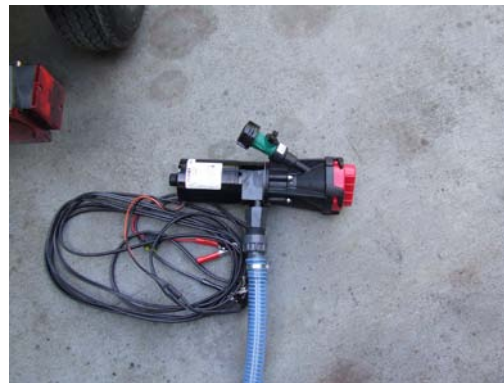
Flow-Jet macerator pump, 1" hose and 20' fused wire harness with switch to attach to a 12v battery. The macerator pump quickly extracts and grinds up the waste from your black and gray tanks and pumps it into the holding tank on the RV TOTE TRAILER.
